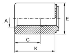
Female thread A = M4Height K = 9Min distance to edge = 4.0Outer diameter E = 8Plate thickness = 0.8 to 1.0
